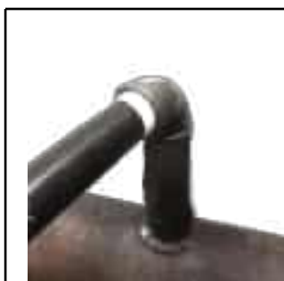
1. Elbow on TOE Nipple
